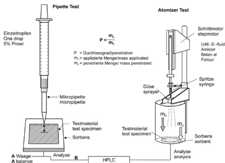
Methods for testing penetration of liquid and dispersed PPP
