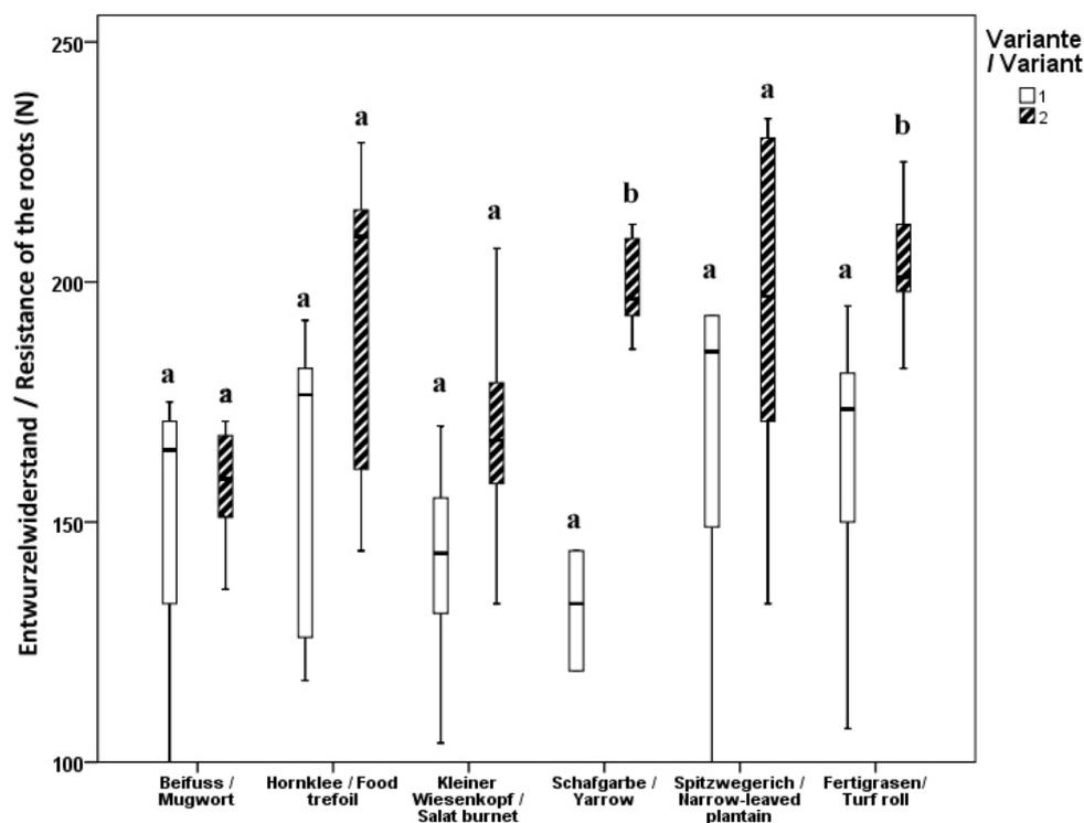
Resistance to uproot in Newton (N), a = dates without significant differences, b = dates with significant differences
