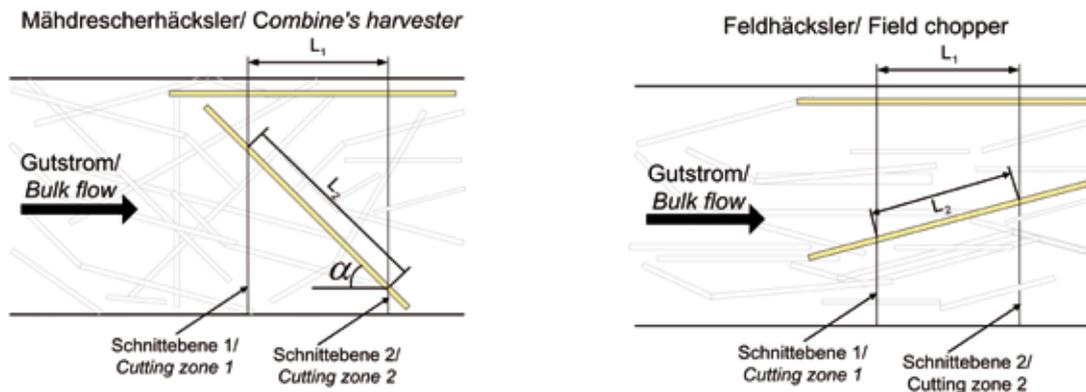
Theoretical and effective cutting length of straw in a combine's harvester and of maize in a field chopper
