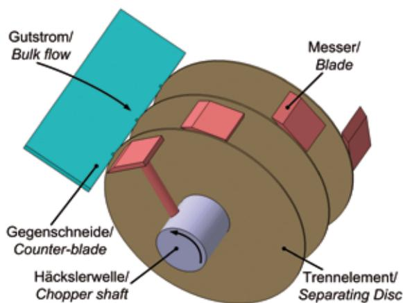
Cutting device with integrated separating discs
