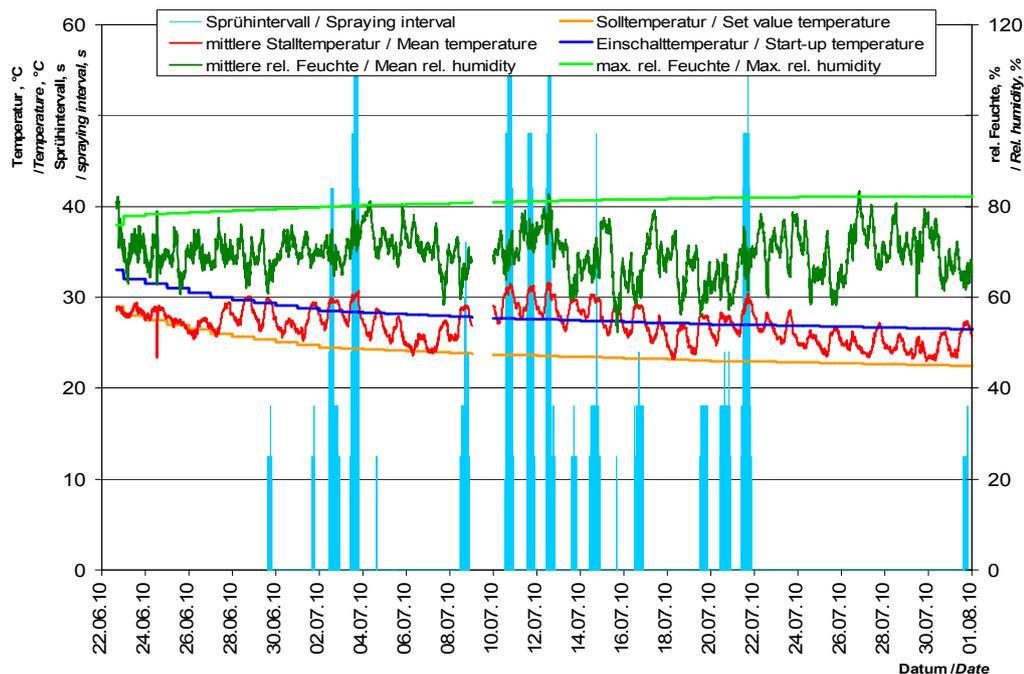
Spraying intervals [s], mean temperature [°C], mean rel. humidity [%] as well as control pattern set value temperature [°C], max. rel. humidity [%] and start-up temperature [°C] for cooling in the period of 22.06.2010 to 01.08.2010
