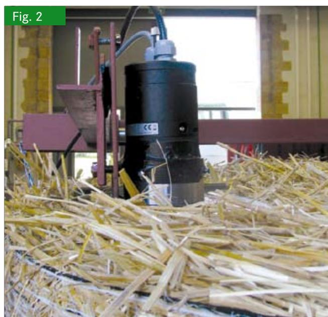
Measuring head installation for radial measurements on bales
