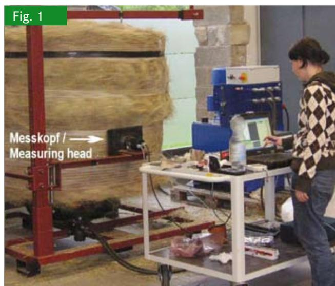
Assembling of test rig with tangential sensor mounting
