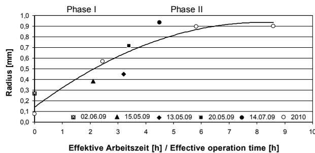
Mean cutting-edge radius as a function of effective operation time during grass silage production in 2009 and 2010
