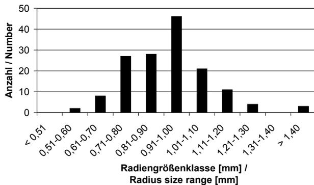
Distribution of the measured cutting-edge radii (14.07.2009, grass, 4.5 h effective operation time)
