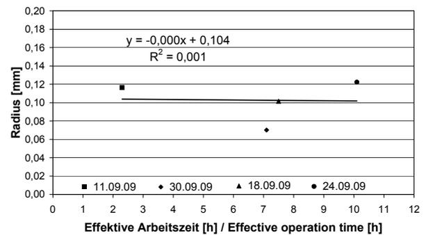
Mean cutting-edge radius as a function of effective operation time during maize silage production in 2009
