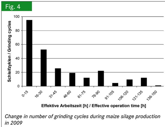
At the start of the maize harvest, the trial forage chopper's driver performed experience-based grinding of his knives in approximately 30 cycles a day (one day = approx. 5 hours of effective operating time). This grinding intensity corresponded to the mean value calculated from a survey of over 100 drivers [5]. Based on his visual inspection of the knives (**figure 5**), the driver continued to reduce the grinding intensity over the course of the harvesting season.
