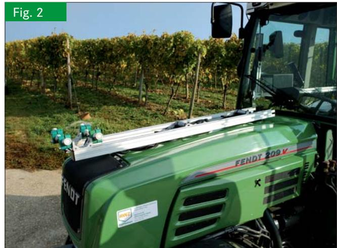
Experimental tractor with mounted ultrasonic sensors
