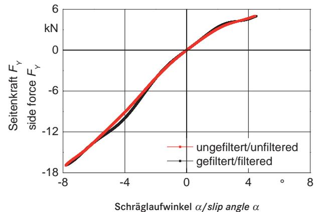
*Side force over slip angle, unfiltered and filtered*
