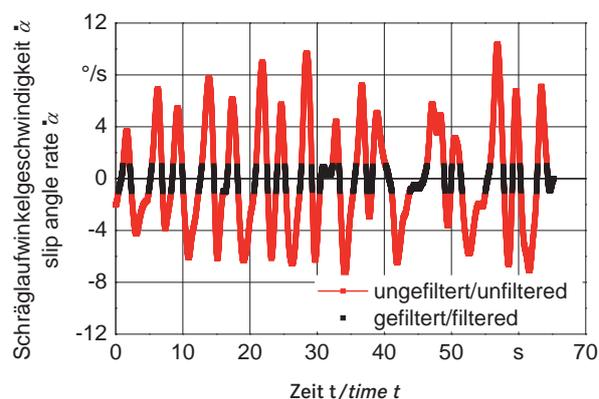
Slip angle rate, unfiltered and filtered
