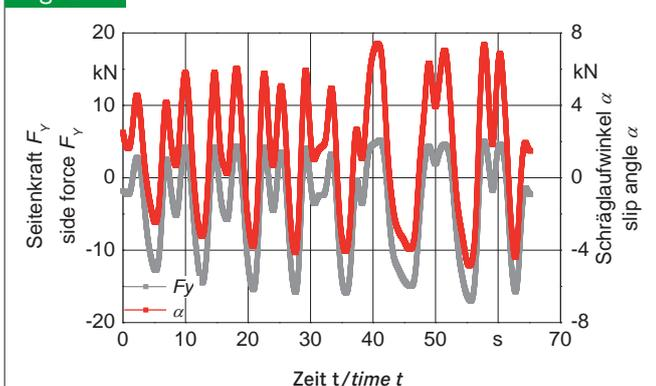
Side force and slip angle at front wheel over time during test run
