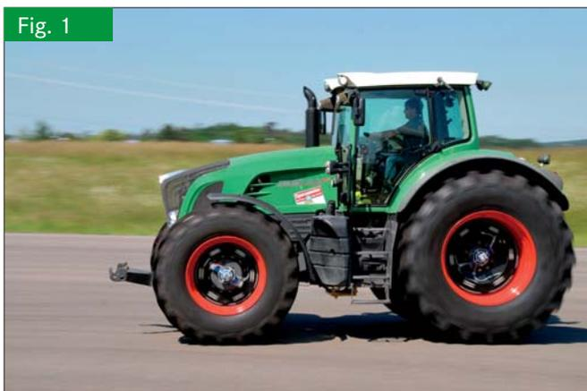
Fendt Vario 936 test machine with Kistler measuring rims
