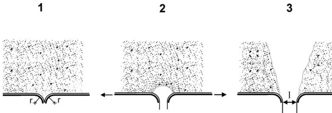
Functional principle of the bridging test apparatus
