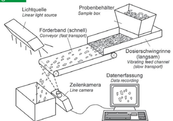
Functioning principle of continuous image analysis
