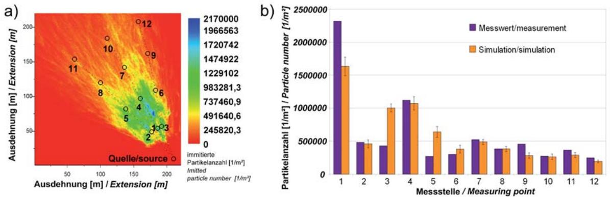
(a) Deposited particle number; (b) Comparison APMS-simulation
