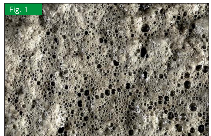
Foam can be a problem in biogas plants. Photo: A. Künzelmann, UFZ
