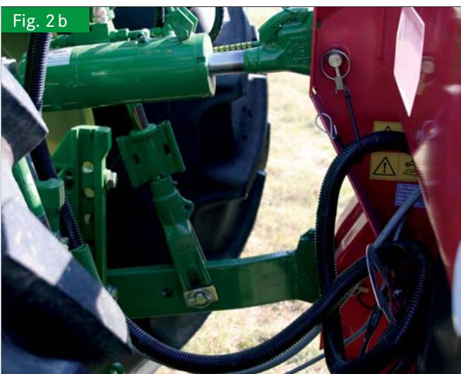
Clearance between tractor and fertilizer spreader
