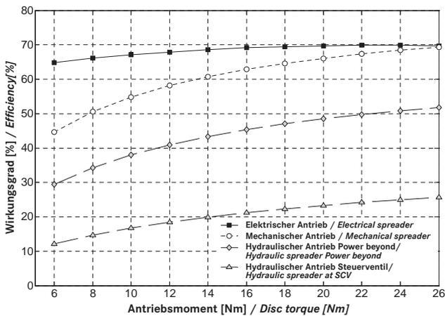
Efficiency of various spreading disc drive systems of fertilizer spreaders [1]
