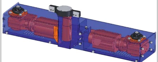
Transparent view of the electrical disc/agitator drive of a fertilizer spreader
