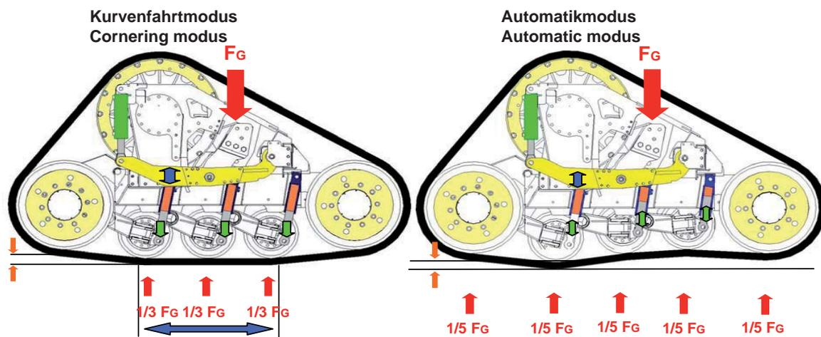
Model of function for suspension, automatic surface alignment and food print reduction.  $F_G$  = load
