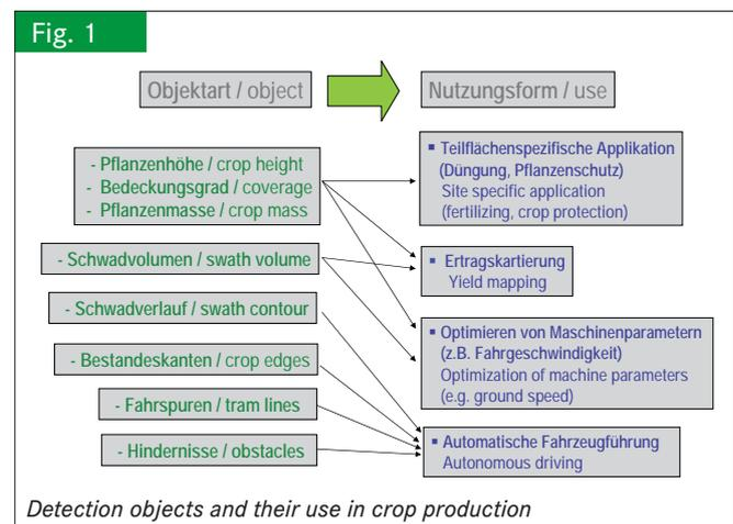
performance and to avoid blockages. Furthermore, the sensor based detection of swath contours, crop stand edges, tram lines, and obstacles can be used to support autonomous driving (auto-guidance) alone or together with satellite based positioning systems.
