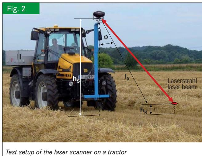
Test setup of the laser scanner on a tractor
