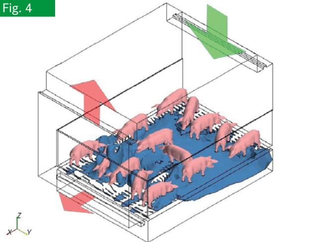
Ammonia cloud of 0.1 ppm in one compartment. Fresh air flows into the room through a channel on the ceiling (above right) and flows out (above left) with substance releases during under-floor suction (bottom left) at the same time. The concentration at the manure surface amounts to 20 ppm (Program STAR-CCM+ from CD-Adapco)
