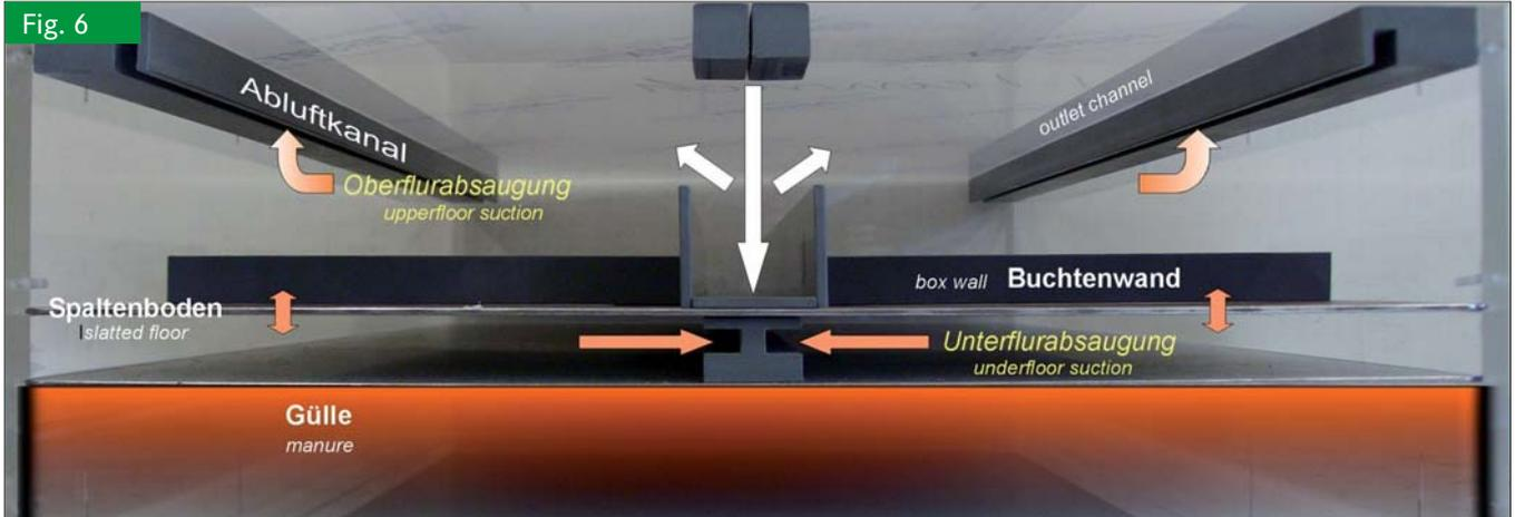
The stable air is drawn into channels on the side walls. Fresh air flows in via an inlet channel at the center of the ceiling. Underneath the slatted floor, the air above the manure is drawn to the centre of the stable and transported to a filter. Because of the width of the slatted floor, it is inevitable that some air is drawn in the room above the floor through the slatted floor
