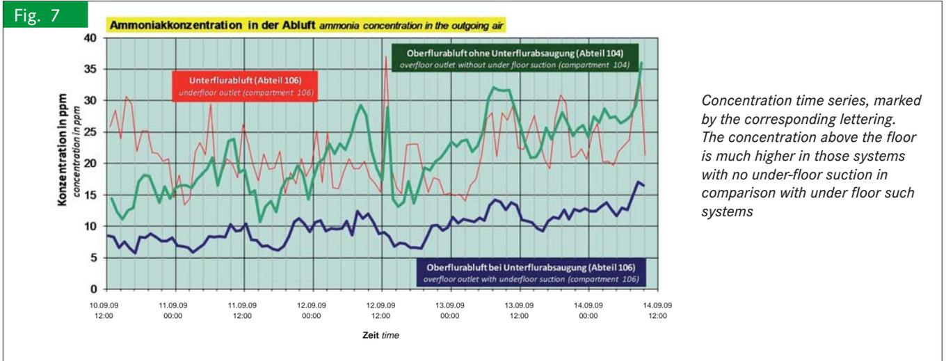
Concentration time series, marked by the corresponding lettering. The concentration above the floor is much higher in those systems with no under-floor suction in comparison with under floor such systems
