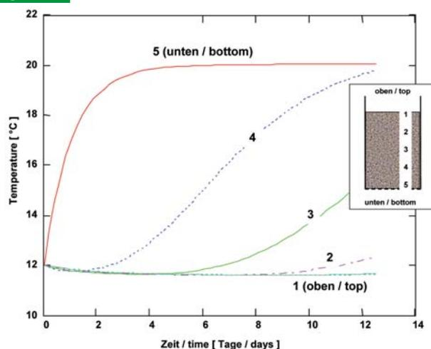
Temperature in wood chips bulk, model; chip size: coarse, non separated
