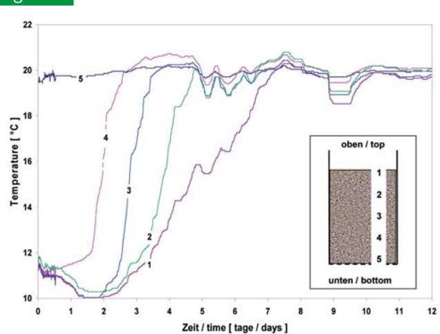
Temperature in wood chips bulk, experiment; chip size: medium, separated
