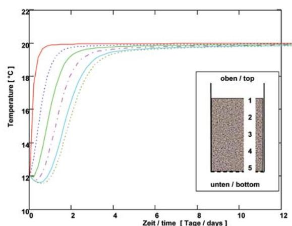
Temperature in wood chips bulk, model; chip size: coarse, separated
