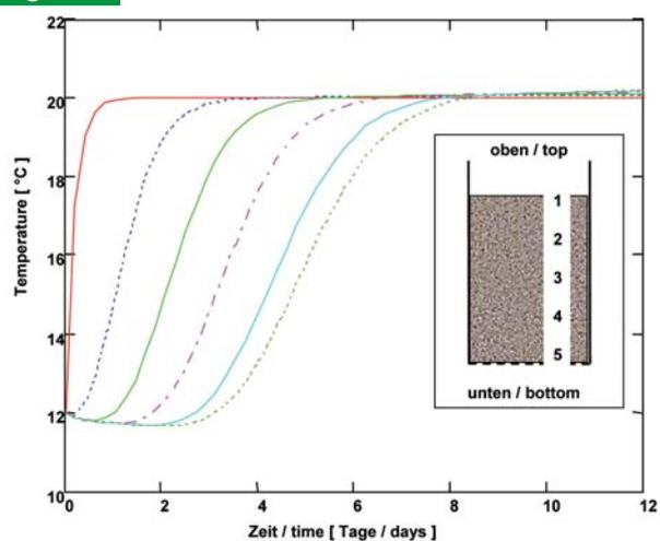
Temperature in wood chips bulk, model; chip size: medium, separated
