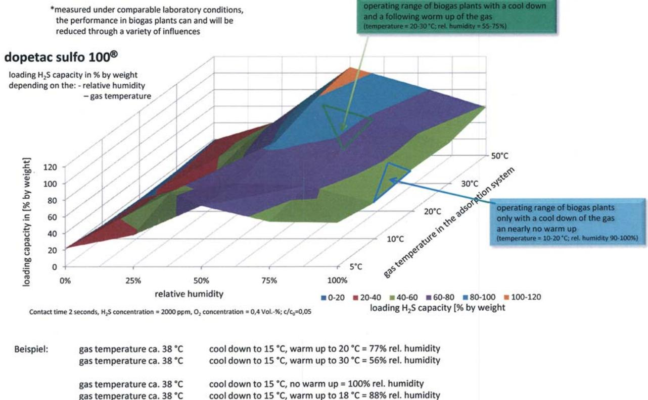
*Laboratory results for the desulfurization capacity with different gas temperatures and relative humidities*
