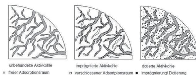
Schematic representation of the pore system of various activated carbons
