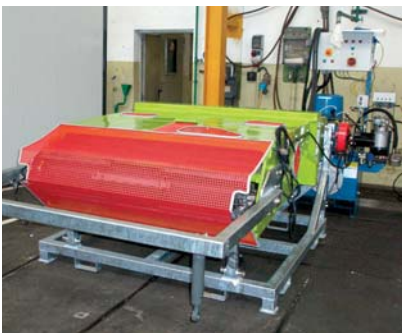
Test stand for feeder house conveyor chain examination
