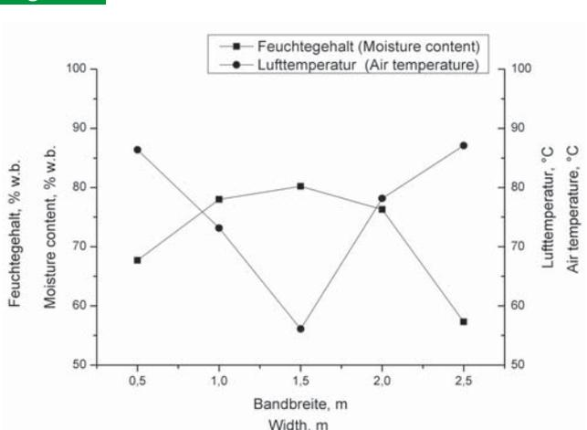
Moisture content and air temperature across the belt width in the middle of the first band
