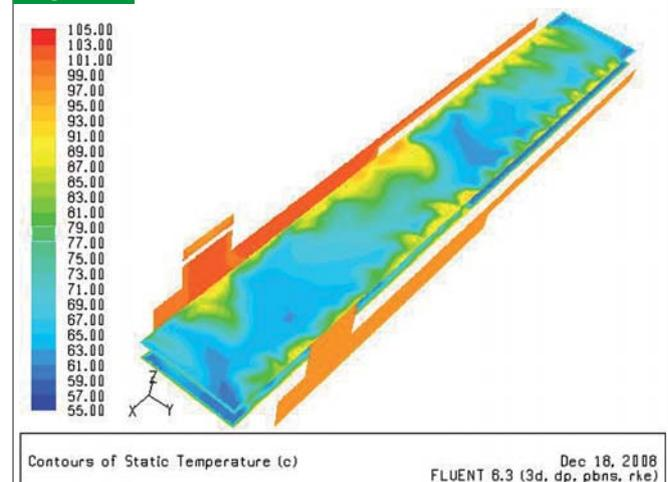
CFD simulation of the temperature distribution above the first dryer band
