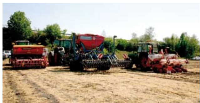
Tested seeding systems (from left: disc seeder, cultivator seeder, single seed drill)
