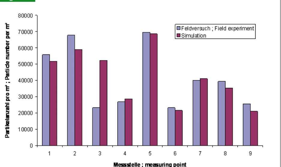
Shown is the number of tracer particles per square meter for each of the nine deposition points. Experimental data is shown in red, while blue shows the simulation results.
