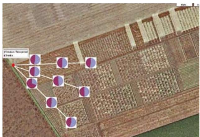
Overview on the experimental area. The red point marks the point of emission, while the pie charts mark the points of dust collecting
