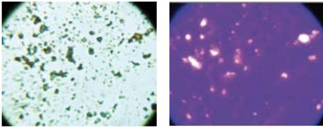
Sample, illuminated with transmitted white light (left) respectively incident ultraviolet light (right)
