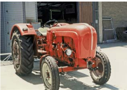
The "Super X" test tractor developed by Porsche featured a stepless hydrostatic transmission.
