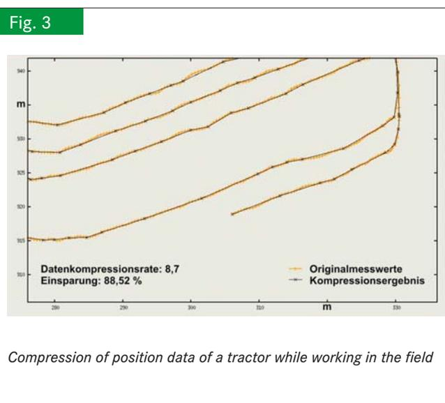
Another example is a method which serves to compress position information determined by the GPS receiver of the experimental tractor during field use. Here, the compression result should also contain only relevant information. However, the necessary relevance criteria are more diverse than in the first example. Figure 3 shows the result of position data compression.
