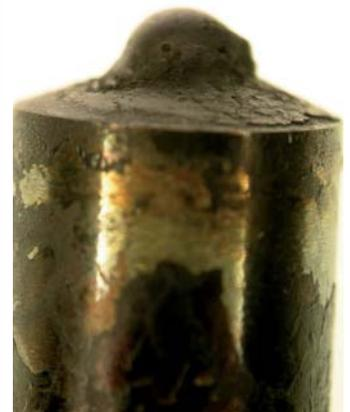
Deposits on the injection nozzle of cylinder 1 of the Fendt Vario 412 after 2653 operating hours
