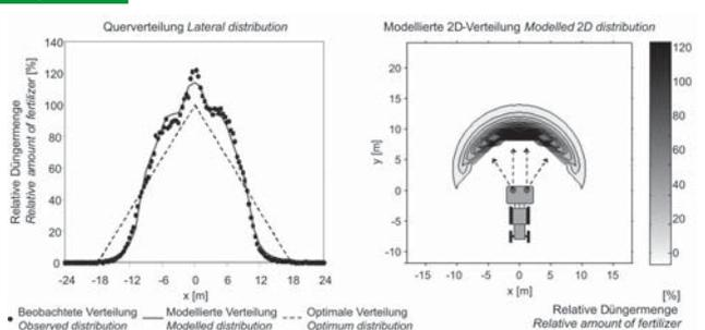
Example of deriving a 2D distribution pattern from a 1D lateral distribution
