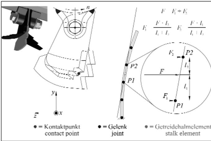
Fig. 2: Determining the contact point, using a chopping knife as an example
