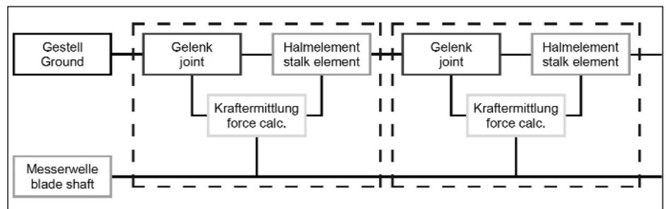
Fig. 4: Structure of a SimMechanics-model for simulating the cutting process
