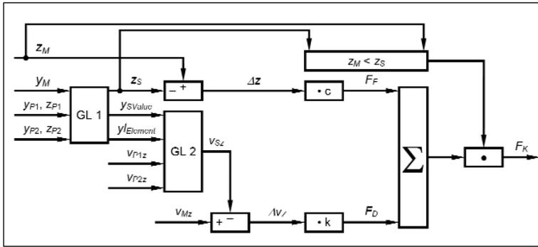
Fig. 5: Structure of a SimMechanics-model for determining the cutting force  $F_K$  (Indexes:  $M$  = knife;  $P1$  and  $P2$  acc. to Fig. 2;  $SK$  = contact point, see Fig. 2;  $x, y, z$  = space coordinates)
