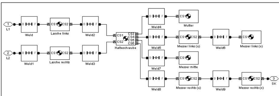
Fig. 3: SimMechanics-model of a knife segment
