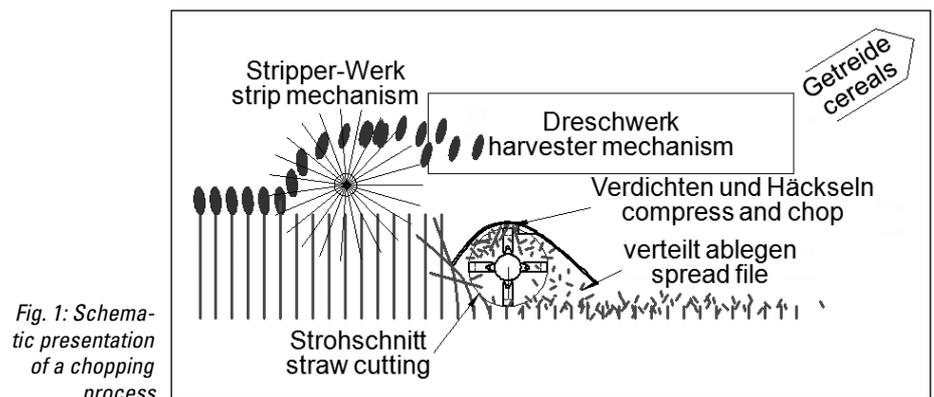
*Fig. 1: Schematic presentation of a chopping process*
