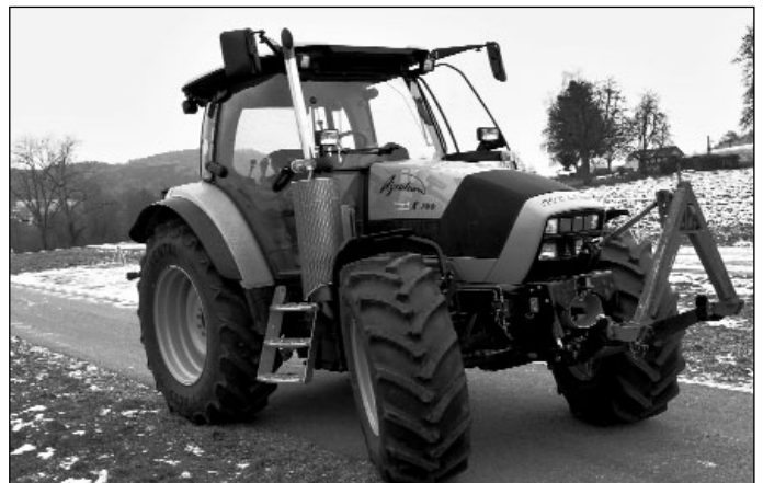
Fig. 1: Tractor retrofitted with a particulate filter
