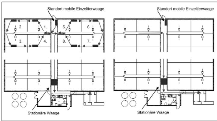
Fig. 1: Ground plan with scheduling for the work processes „weighing with mobile single animal scale“ (left) and for „weighing with a fixed scale“ (right) in a pig fattening house with 1600 fattening places, 10 compartments each with 4 pens and 40 pigs per pen [7]
