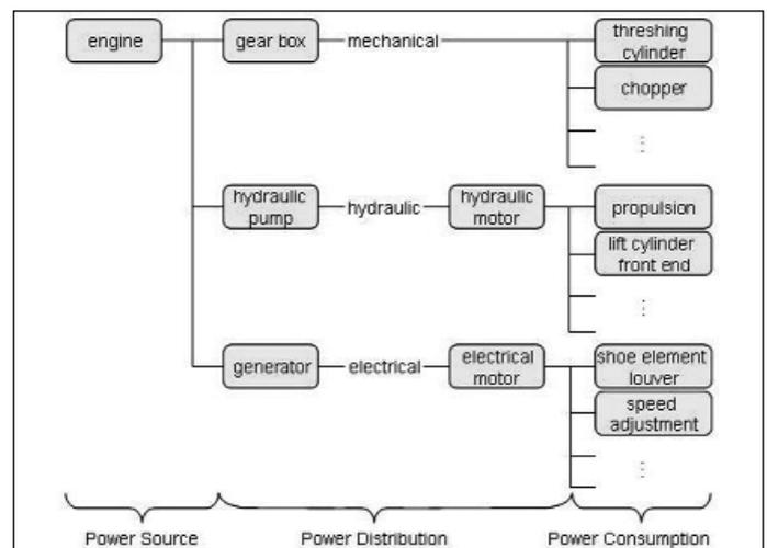
Fig. 1: Schematic power split in a combine harvester
