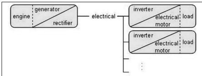
Fig. 2: Electrical powertrain in a combine harvester
