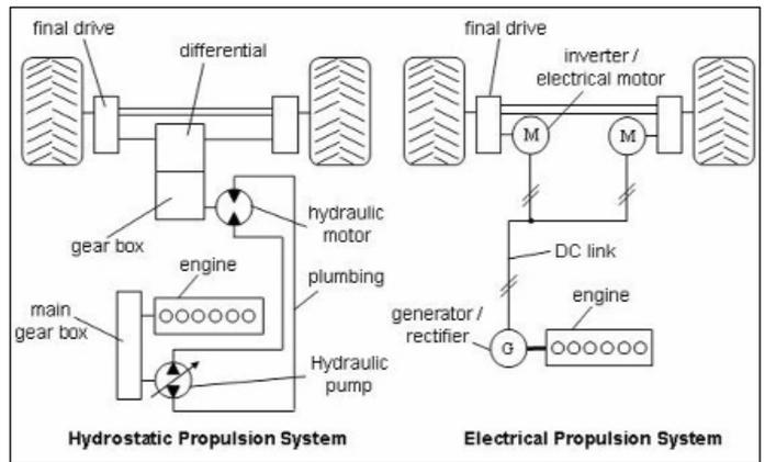
Fig. 3: Hydrostatic and electrical propulsion in a combine harvester
