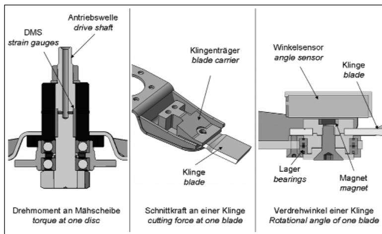
*Fig. 1: Measuring technology used*
