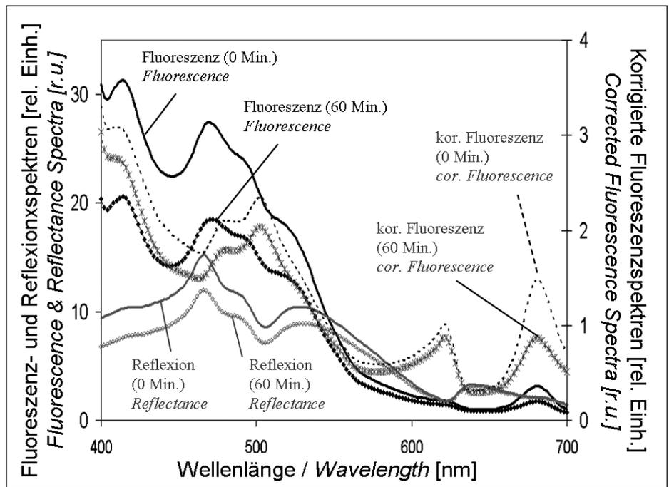
Fig. 2: Fruit fluorescence spectra, diffuse reflectance spectra, and relative fluorescence spectra measured on the fruit tissue, directly after cutting the apple (0 minutes) and 60 minutes later
