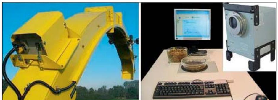
Fig. 1: “HarvestLab™”-sensor mounted on a forage harvester and in stationary set-up
