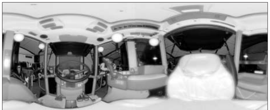
Fig. 1: Two-dimensional illustration of the primary scan from the driver seat view
