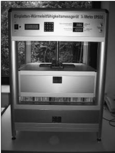
Fig. 2: Measuring the thermal conductivity
