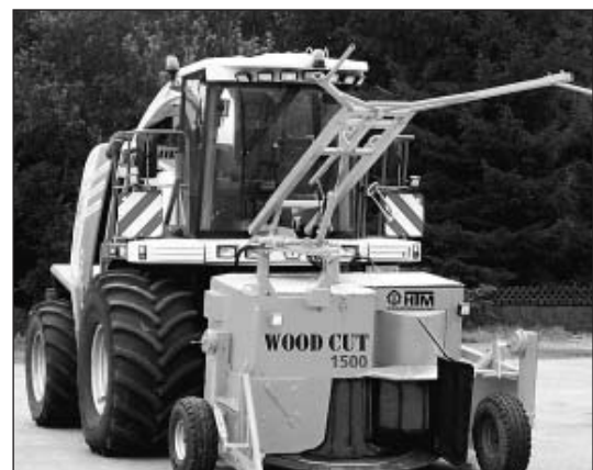
Fig. 1: The new screw chipper WoodCut by HTM, attached to a Big X
