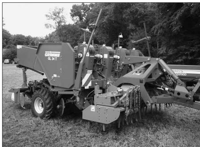
Fig. 1: The GL 34T from Grimme allows tillage, potato planting, and ridging to be carried out in one pass (photo: Dr. Metzner)
