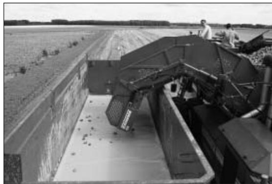
*Fig. 3: In the new Varitron 270 from Grimme, great importance was attached to gentle delivery of the harvested potatoes (company photo)*
