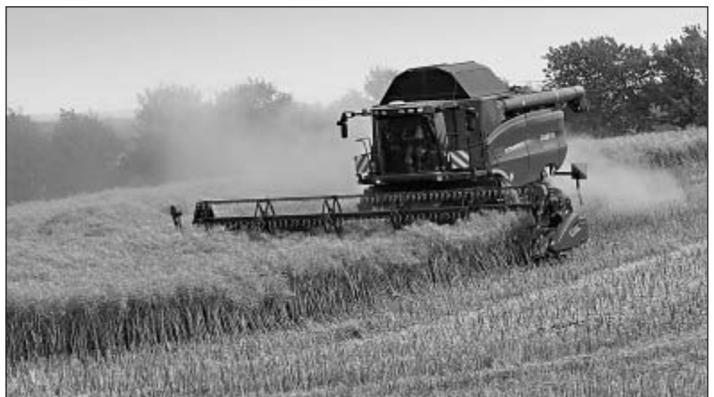
Fig. 2: In its new Axial Flow 9010, Case uses a small tube rotor, which is particularly advantageous for moist and tough crops (company photo).
