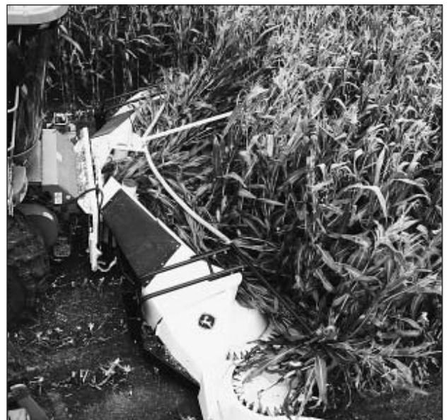
*Fig. 3: Kemper has developed the row-independent cutting head Champion 475 for the harvest of high-yielding energy maize*
