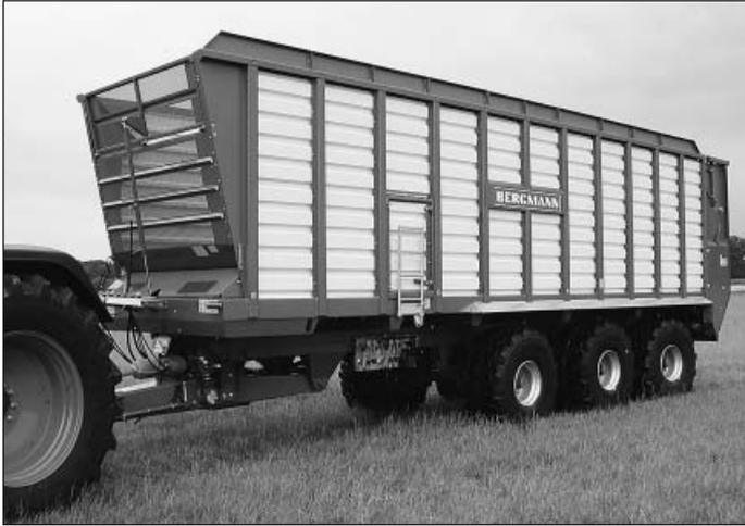
*Fig. 2: Bergmann has adjusted its trailer HTW 65 for chopped forage to the increased capacities of the forage harvesters: 65 m<sup>3</sup> loading volume and a hydraulic Tridem travelling gear are the insignia.*
