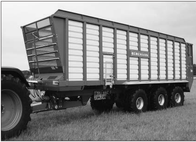
Fig. 2: Bergmann has adjusted its trailer HTW 65 for chopped forage to the increased capacities of the forage harvesters: 65 m 3 loading volume and a hydraulic tridem travelling gear are the insignia
