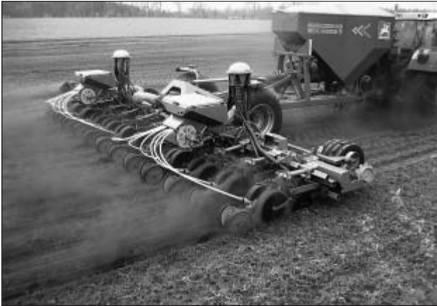
Fig. 2: In its space drill EDX 9000-T, Amazone separates seed singling and the placement system and thus realizes working speeds of up to 15 km/h.
