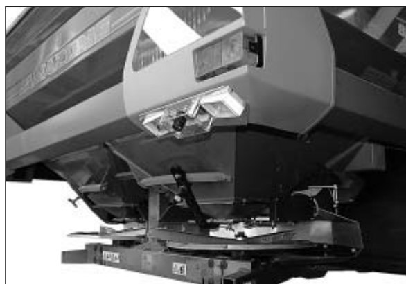
Fig. 3: The camera system Argus from Amazone allows for contactless scanning of the spread fan in order to determine the set values of lateral distribution (company photos)
