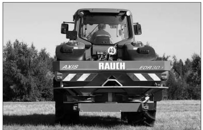
Fig. 4: Rauch drives its two-disc fertilizer spreader electrically, which provides precise fertilizer distribution, low energy input, and high operating comfort.
