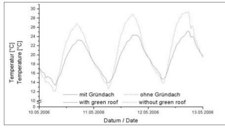
Fig. 1: Profile of daily temperature measures inside the stable of the green roof and roof without plants in May 2006
