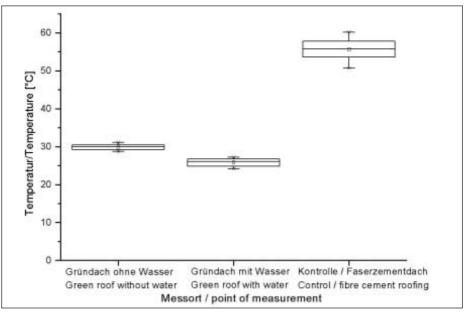
*Fig. 2: Distribution of temperature measures at the bottom side of the green roof compared to control without green roof*
