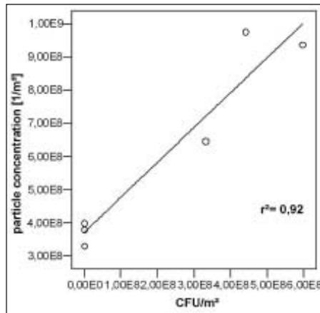
Fig. 4: Relationship between the total dust particles and the mould spores collected with the GSP in the dust releasing cube
