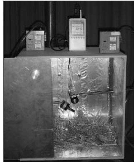
Fig. 1: Dust releasing cube with a PGP-GSP and -FSP measuring apparatus and the climatic console
