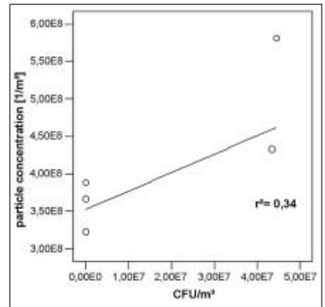
Fig. 5: Relationship between PM 5 and the mould spores collected with the FSP in the dust releasing cube
