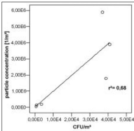
Fig. 3: Relationship between the total dust particles and the mould spores collected with the GSP in the selected measurements
