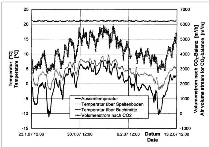
Fig.2: Typical course of temperature outside and inside the pig-fattening house as well as air volume flow in winter
