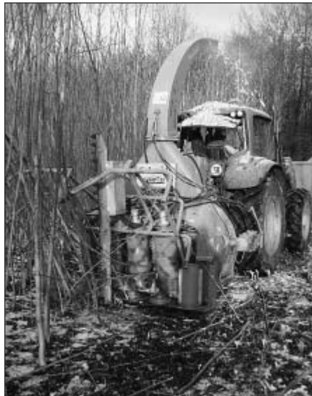
Fig. 1: Young growth chopping of ash in an overgrown scattered orchard meadow with the new prototype of the landscape conservation chopper
