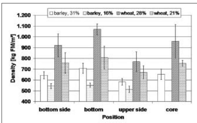
Fig. 2: Density of crimped barley and wheat with different moisture contents (W.B.) at various positions within the silage bag
