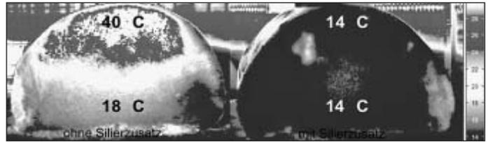
Fig. 3: Thermography picture of barley in the silage bag with 31% moisture content (W.B.). Left: Intensive secondary fermentation of the control variant; right: secondary fermentation can be decelerated significantly with a chemical additive
