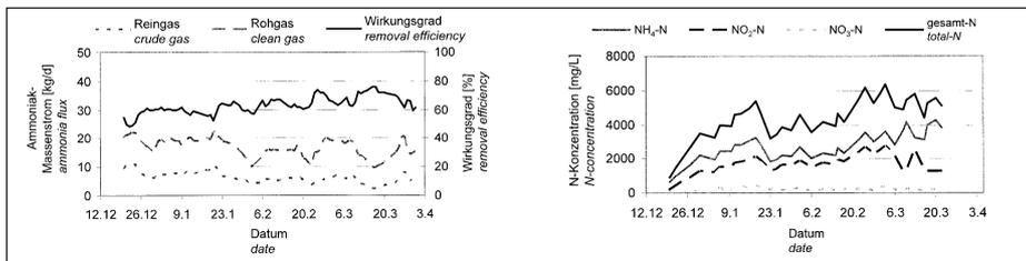
Fig. 2: Left: Ammonia mass flow and removal efficiency of the 2<sup>nd</sup> biological experiment with ground water. Right: Developing of ammonia-, nitrite- and nitrate concentration as well as total N-concentration during the 2<sup>nd</sup> biological experiment with ground water
