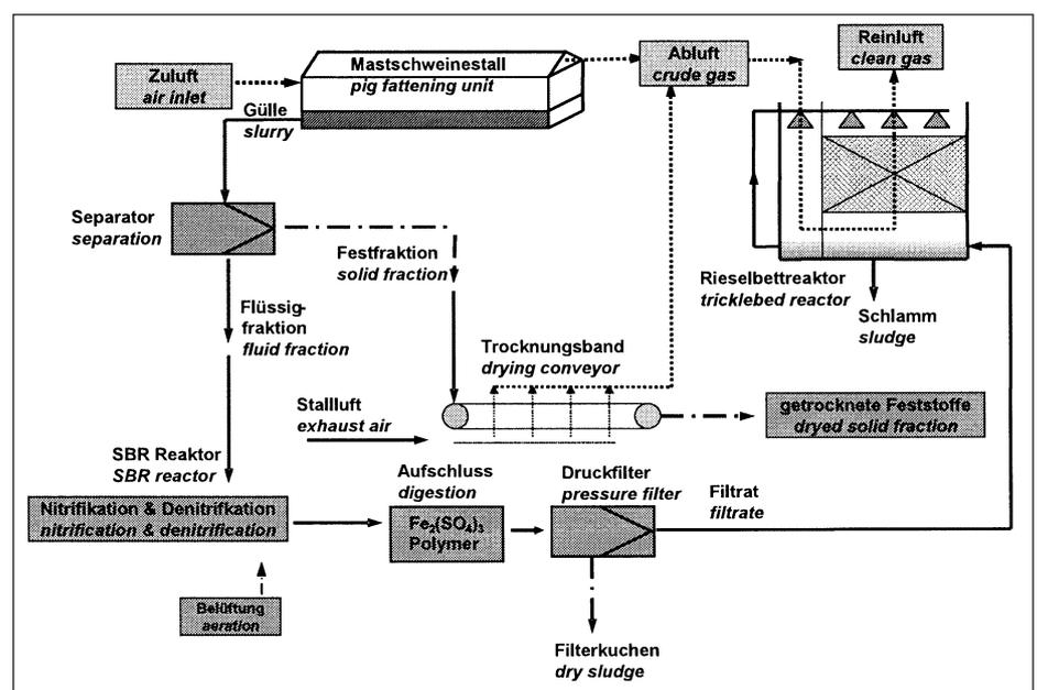
Fig. 1: Process flow of the Ecowel<sup>®</sup> Farm-System (Fa. WEDA)
