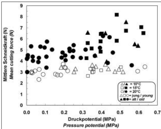
Fig. 3: Effects of pressure potential on the mean cutting force of young and old radish tubers, obtained at 10, 15 and 20°C
