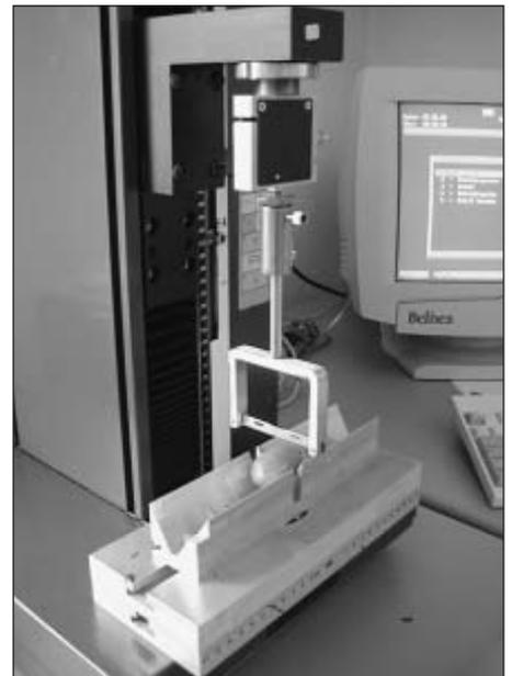
Fig. 1: For cutting, a microtome blade (Feather S35, 0.26 mm thickness), adapted to the universal testing machine (Zwicki 1120, Zwick GmbH & Co. KG, Germany) was used.
