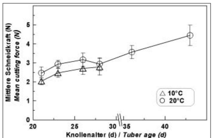
Fig. 4: Effects of differentiation on the mean cutting force as obtained at radish tuber temperatures of 10 and 20°C
