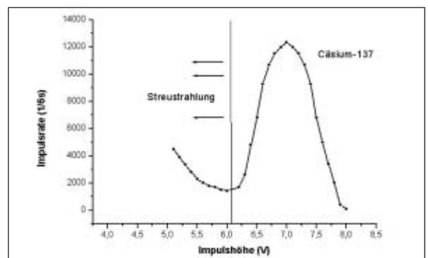
Fig. 1: Gamma energy spectrum of Caesium<sup>137</sup> with discriminatory voltage of ~ 6 V
