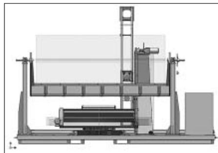
Fig. 4: Mobile density test stand of the DLG for bilateral irradiation of round and square bales
