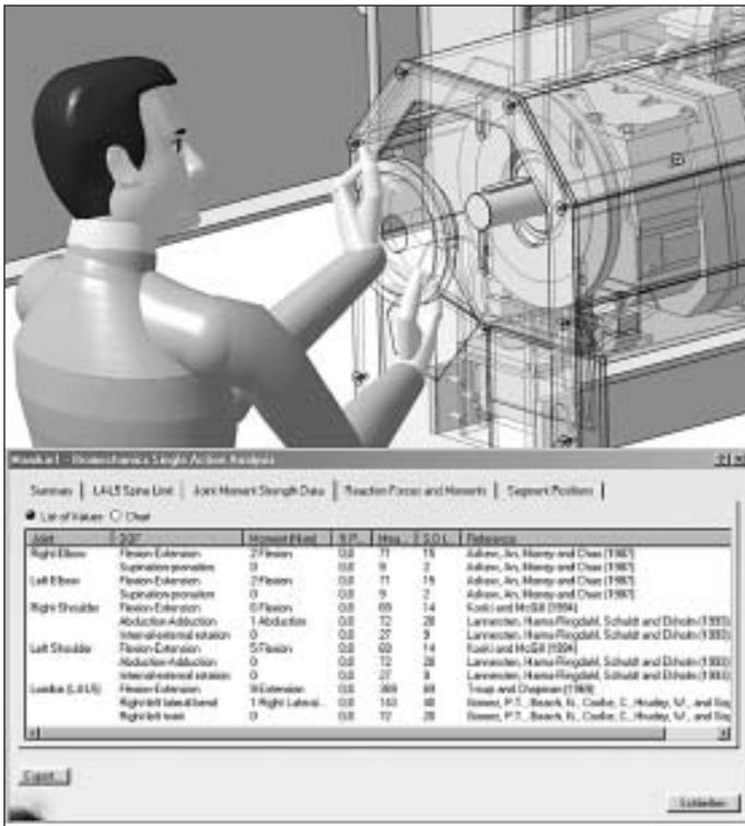
Fig. 2: Assembly simulation with analysis of the biomechanical stresses
