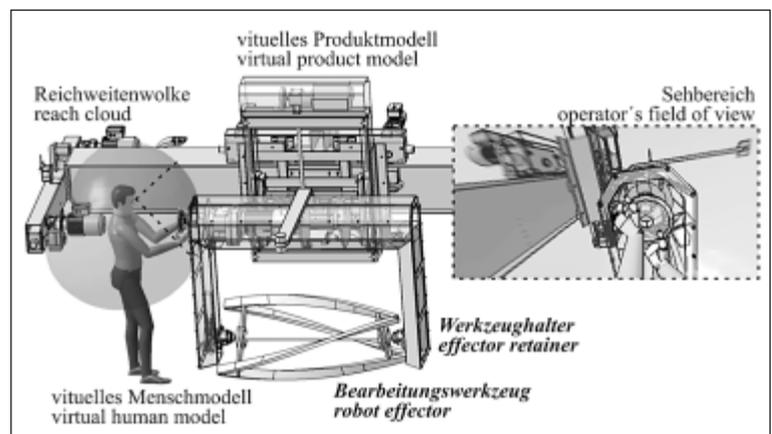
Fig. 1: Virtual product model of the mixing and transporting robot
