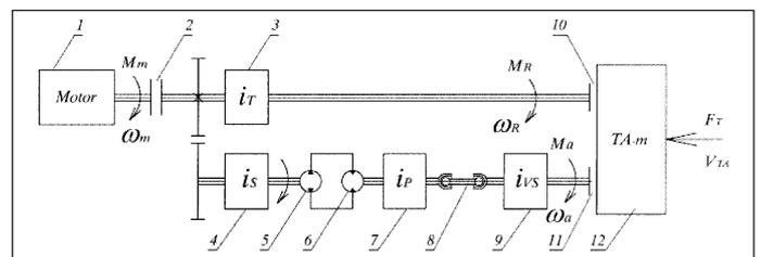
Fig. 2: The hydraulic circuit for the trailer drive
