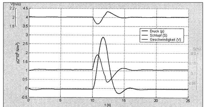
Fig. 5: Result of a simulation calculation: jump of  $\mu_{max} = 0.8$  to  $\mu_{max} = 0.3$
