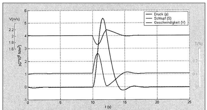
Fig. 4: Result of a simulation calculation: jump from  $\mu_{max} = 0.8$  to  $\mu_{max} = 0.5$
